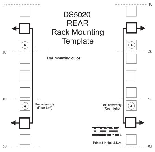
Figure 90. Rear rack mounting template
